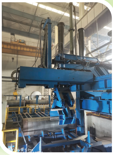
Hot rolling adding automatic sleeve loading equipment
