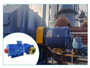
Permanent Magnet-Gear Drive System
