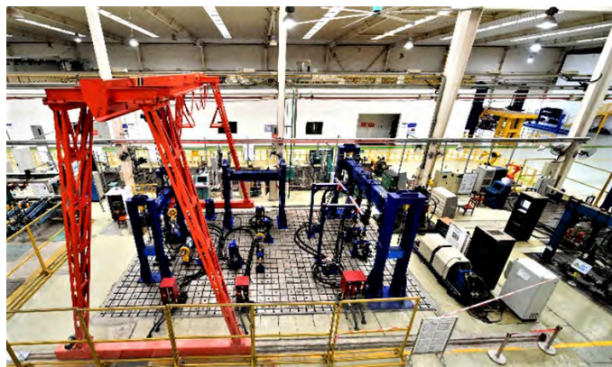
Six-channel comprehensive fatigue test bench 六通道綜合疲勞試驗台
