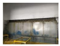
Water Curtain System for collection of spray paint exhaust
