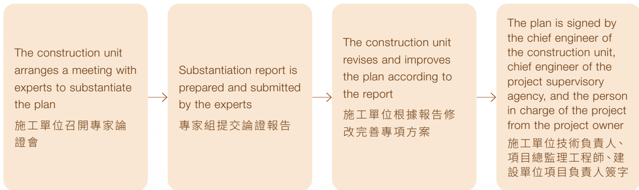
Process of formulating special plans for sub-projects exceeding a certain scale with significant risks 超過一定規模的較大危險性分部分項工程專項方案制定流程
