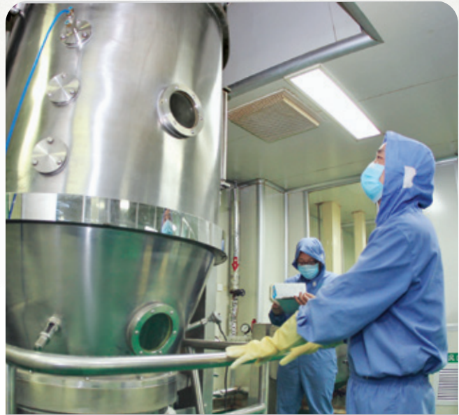
陝西紫光辰濟藥業有限公司顆粒一步製粒 One-step granulation of granules in Shaanxi Unisplendour Life Care Pharmaceutical Co., Ltd.*
