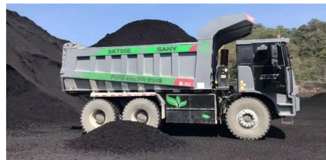
Figure: SKT90E, the first pure electric wide-body loader
