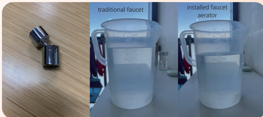
The amount of water flowing from an aerator faucet compared to a traditional faucet after 30 seconds
