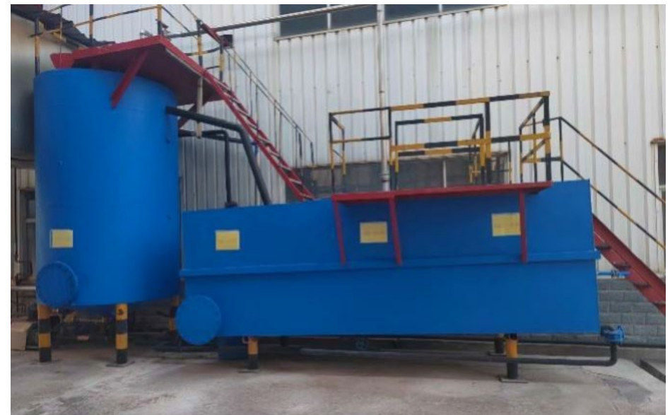
> Waste diatomaceous earth recycling equipment
