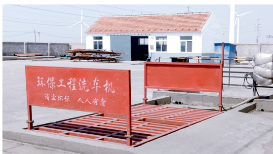
Vehicles washing machine 洗車機
