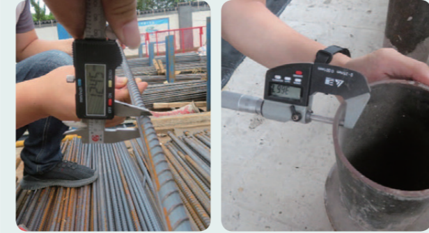
鋼筋直徑、預埋管壁厚測量 Measuring the diameter of steel bars and the thickness of embedded pipes
