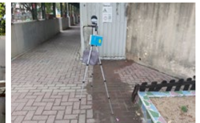
Sound level meter used for measuring the sound created from site to control the noise level
