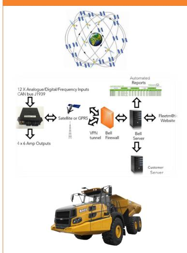
The Bell brand dump truck installed with Fleetm@tic® is a satellite-based fleet management system that provides automated reports, alerts, production data, various packages to choose from and pole-to-pole satellite coverage to keep track of the equipment at the worksites on a continuous basis. This allows customers to manage their fleet with precision, and overall greater enhances operational efficiency.
