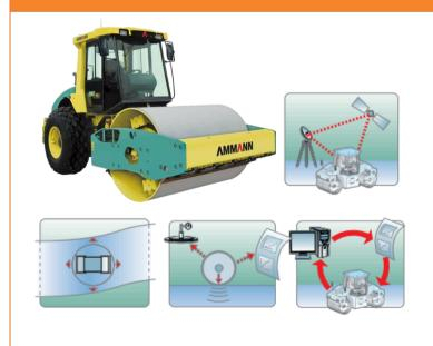
The Ammann Compaction Expert (ACE), a proprietary intelligent compaction system installed in Ammann brand rollers, is able to provide data regarding the areas the roller has covered through GPS mapping capabilities.
