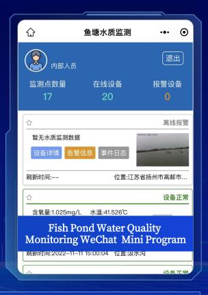
Once the results of indicators such as dissolved oxygen and water temperature are detected as Abnormal, fisher farmers get alerts in the first place. Meanwhile, devices for increasing oxygen level are triggered jointly for rapidly improving water quality and preventing death of large quantities of the subject matters.
