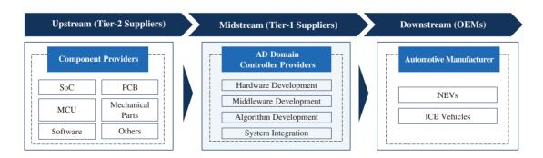
Upstream participants, such as Mobileye, are Tier-2 suppliers for components of AD domain controllers, such as SoC, MCU, PCB, and software, with SoC being the most important and valuable component that is directly related to the performance of an AD domain controller.
