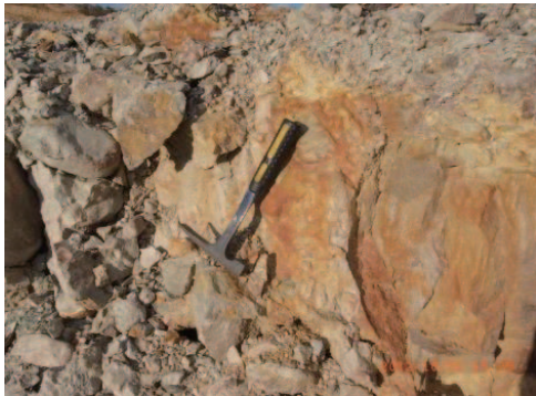
Partly oxidised mineralised conglomerate
