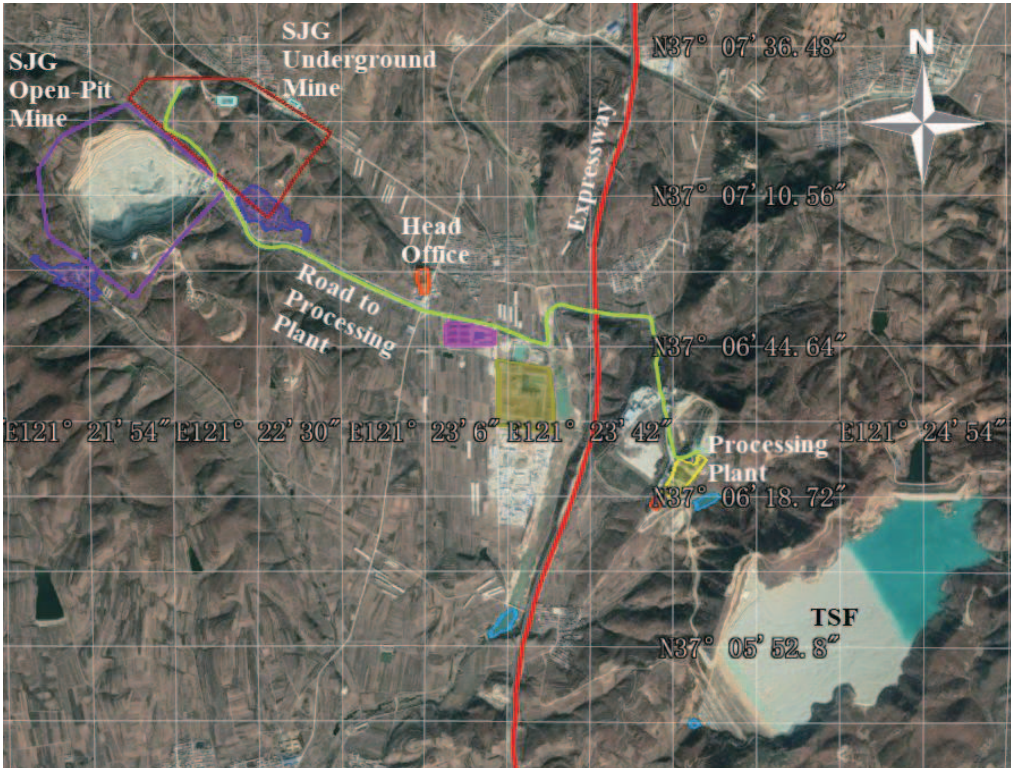
Figure 16-2: Simplified General Layout of SJG Project
