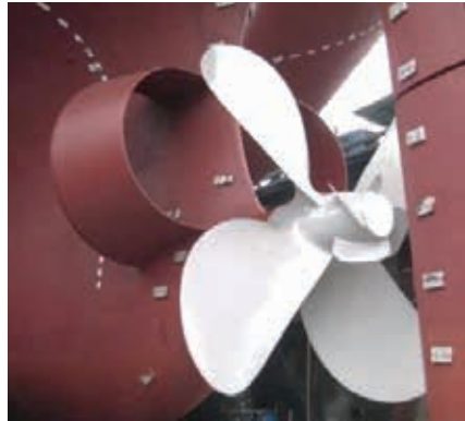
Photos showing pre-swirl vanes (PSV) and Mewis ducts, propeller boss cap fins and a silicone painted propeller
