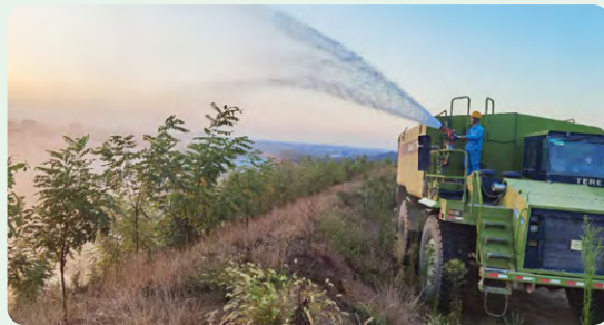
Mine cars sprinkle water to suppress dust
