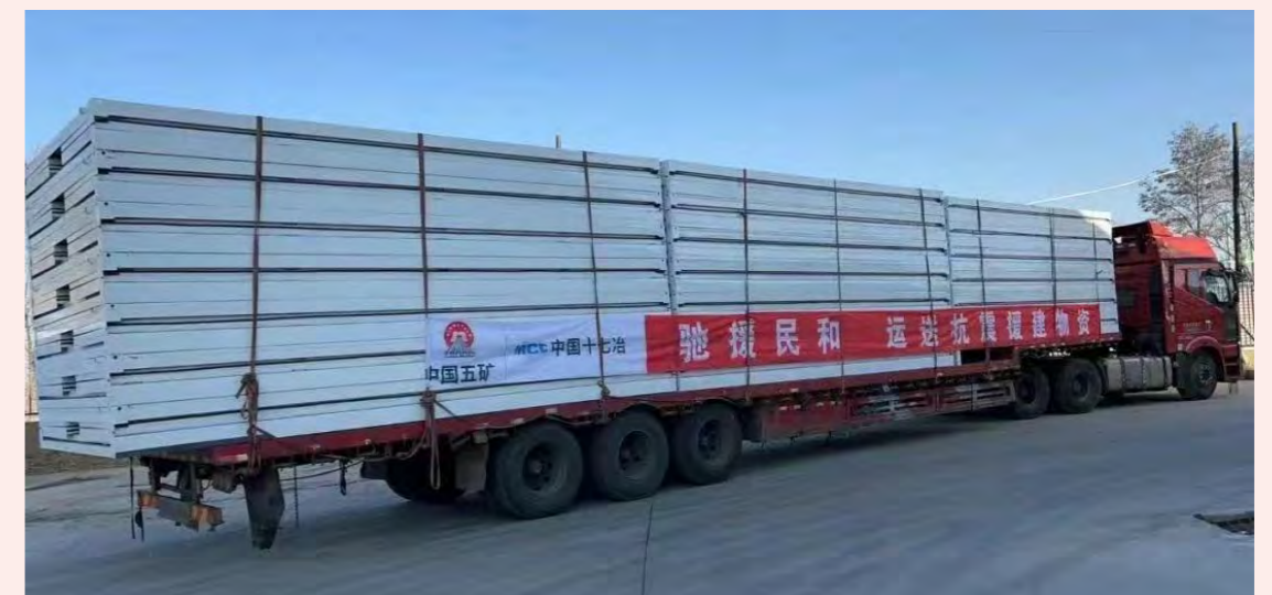
Materials of prefabricated houses loaded for transport
