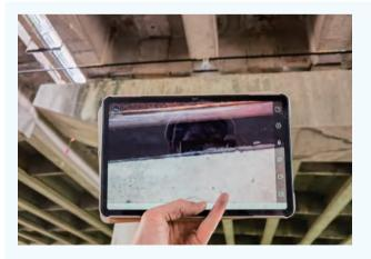
Ningbo Management Centre developed intelligent inspection device for bridge bearings, which ensures the accuracy of the inspection while improving the inspection efficiency and reducing the operational risk.
