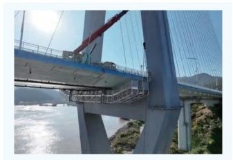
Zhoushan Management Centre put into use a new type of girder bottom inspection vehicle at the Taoyaomen Bridge, which adopts fully automatic control and has the characteristics of accuracy, safety, environmental protection, no noise and no pollution.
