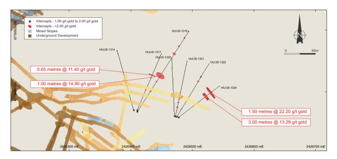
Figure 6 – Arpola-1 2024 Drill Hole Plan.
