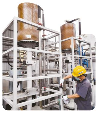
Waste oil recycling using VMAT technology
