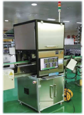
Utility model patent certificate, software copyright certificate and independently developed equipment of the online intelligent vision detection system of milk powder cans
