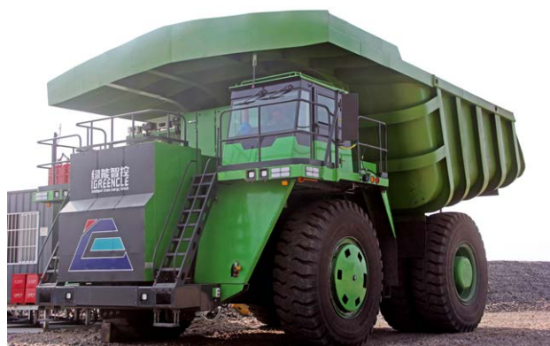
Pingshuo Group’s first 120-tonne chargeable mine truck was put into operation
