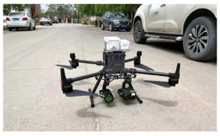
Unmanned Natural Gas Leakage Patrolling Detection System
