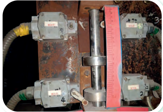
Figure 4: Shift from two swing arm travel switches to three firing pin travel switches
