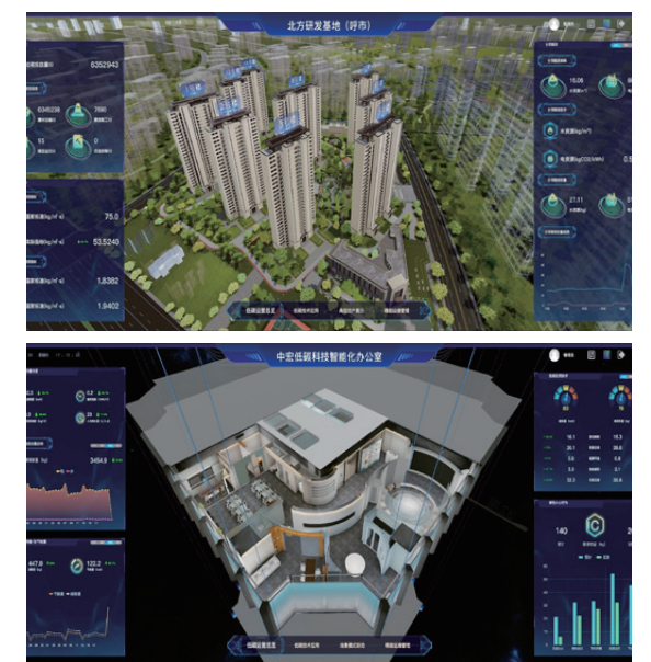
Dashboard of the digital twin energy consumption monitoring platform
