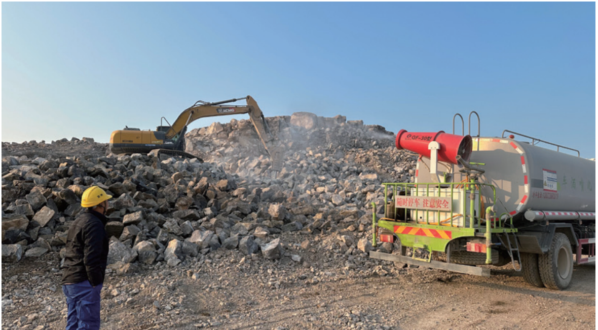
The mining excavator and crushing machinery using fog cannon to reduce dust, with one cannon for each machinery
