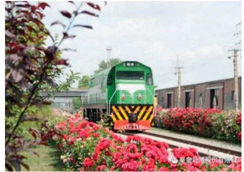
The first pure electric shunting locomotive transformed from an old diesel locomotive in China
