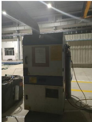
Movable Welding Smoke Treatment Facilities
