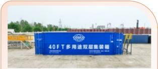
The first dual-layer, multi-purpose container, co-developed by DFIC Qidong and Shanghai PANASIA Shipping Co., Ltd., has been successfully launched. This container can accommodate four cars. It comes with detachable ramp boards for transporting vehicles of various wheelbases, and supports most family car models, which significantly enhances the loading efficiency. For return voyages, it can carry bulk cargo like pulp, improving transportation efficiency while reducing costs.
