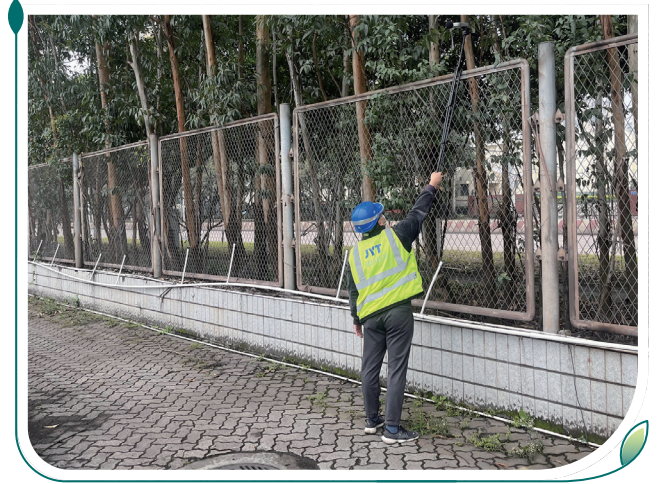
Noise monitoring at Zhangzhou Port
