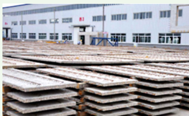
Prefabricated floor slabs
