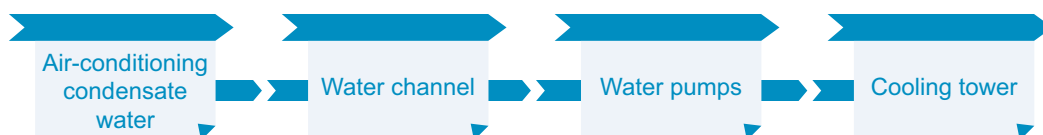
Air-conditioning Condensate Water Reuse Process Design
