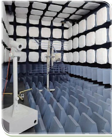
Fully Anechoic 3 meters Chamber 3米法全電波暗室
