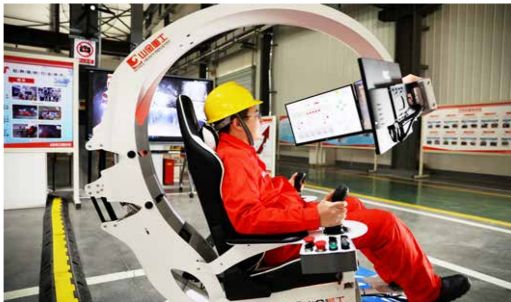
The remote control of large trackless mining equipment based on WiFi6 Mesh, the first of its kind, was tested successfully at Sizhuang Site of Jiaojia Gold Mine. Therefore, the remote control of trackless mining equipment was realized.
