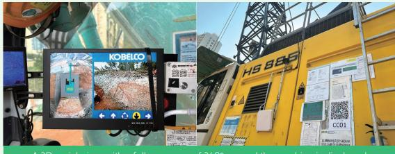
A 3D aerial-view with a full coverage of 360° around the machine is displayed
