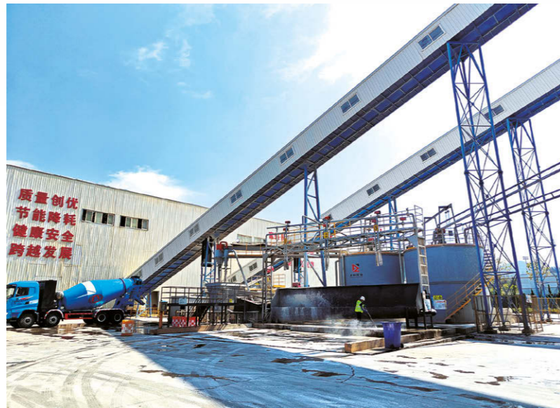
Application site drawing of sand and stone separation + slurry water mixing recycling system
