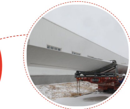
The team of DEC Wind Turbine Manufacturing Project checked the pre-tightening parts of the wind turbine blades at DEC Xing'an League Wind Power Base
