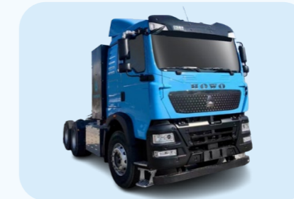
HOWO TX/423kWh/central driving/rechargeable tractor
