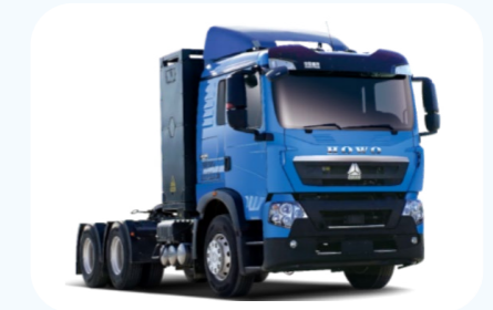
HOWO TX/350kWh/central driving/battery-replacement tractor
