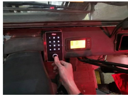
"Seat belt-fingerprint interlocking" device
