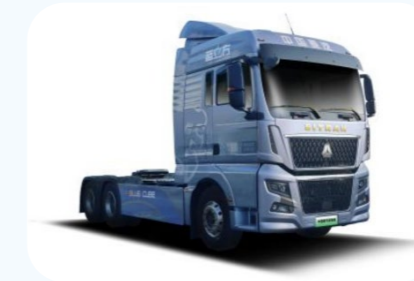
SITRAK GX/513kWh/tractor with electric driving axles and chassis battery-replacement
