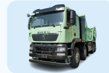
HOWO TX/423kWh/central driving/rechargeable dump truck
