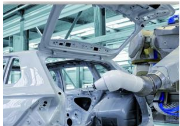
Automatic Coating Robot
