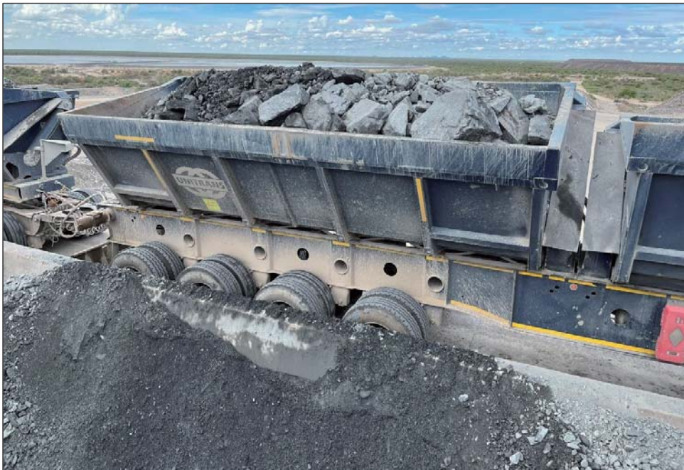
Figure 11-14 Side-tipping ore haulage at the Boseto Plant Source: ERM, 2023
