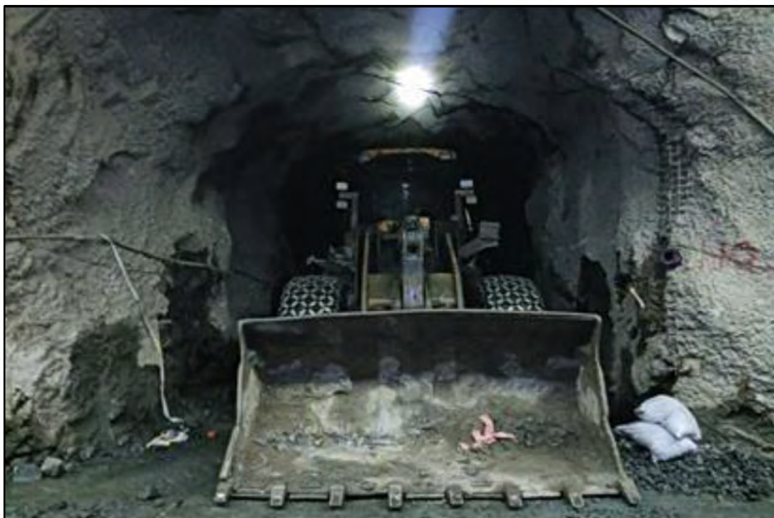
Figure 15-7 Front-end loader at ore pass.
