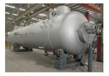
Low pressure water sealed tank
