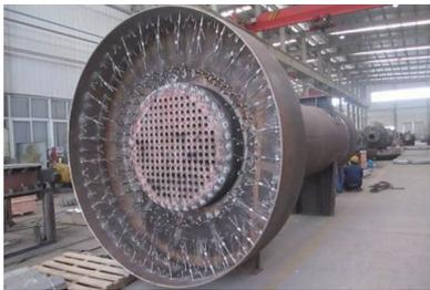
Waste heat boiler is a fire tube boiler connected to heat reactors used in SRUs. It mainly serves to recover high heat by producing medium pressure steam and cool down the gas during the process.
