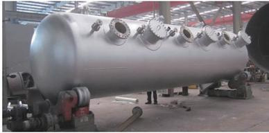
Catalysing reactor is responsible for boosting catalytic effect in order to decompose and turn organic sulphur compound such as carbonyl sulfide and carbon disulfide into hydrogen sulfide and carbon dioxide.
