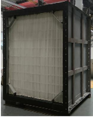
The product's core is made of modified polymer plates and the shell is made of metal with anti-corrosion coating. It is mostly used in flue gas de-whitening projects. Compared with material such as metal and glass, plate form polymer phase transition agglomerator is compact and lightweight, and is resistance to acidic corrosion of sulfur and nitrogen-containing compounds.
