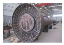
Waste heat boiler is a fire tube boiler connected to heat reactors used in SRUs. It mainly serves to recover high heat by producing medium pressure steam and cool down the gas during the process.
