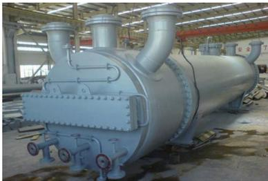
Sulphur condenser forms the shell and tube boiler of a special type of heat exchanger. The main function is to cool down sulphur generated in the upstream reaction section of heat exchanger systems.
