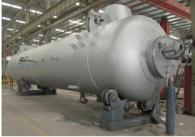
*Low pressure water sealed tank*
