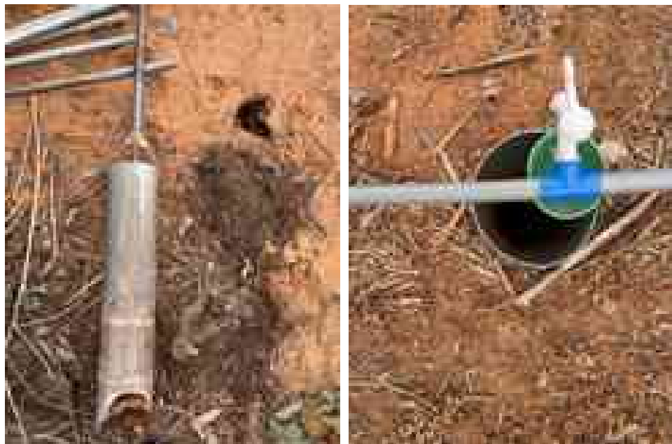
Figure 12-6: Auger and Injection Hole
