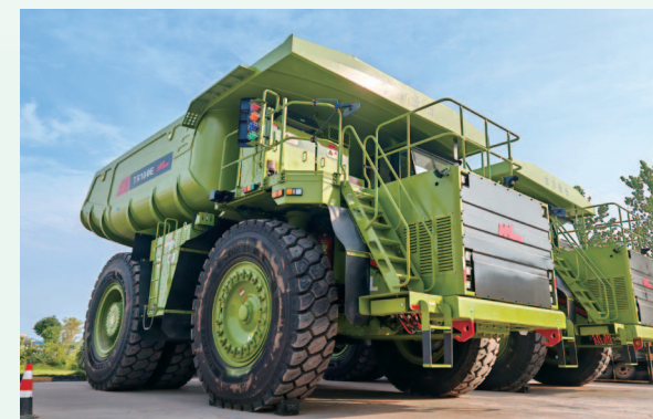
Zongyang Conch TR100E electric mining truck
