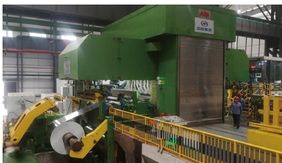
Development and application of six-roll cold rolling equipment for 2,800mm wide high-precision aluminium alloy sheet and strip
