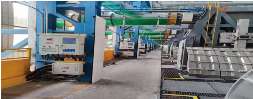
Multi-parameter balance control technology and equipment for aluminum electrolysis cells
