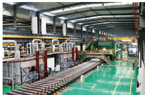
Key technology and equipment development for the 3,300/2,800 twinstand aluminum plate and strip hot rolling mill (1+1 production line)
