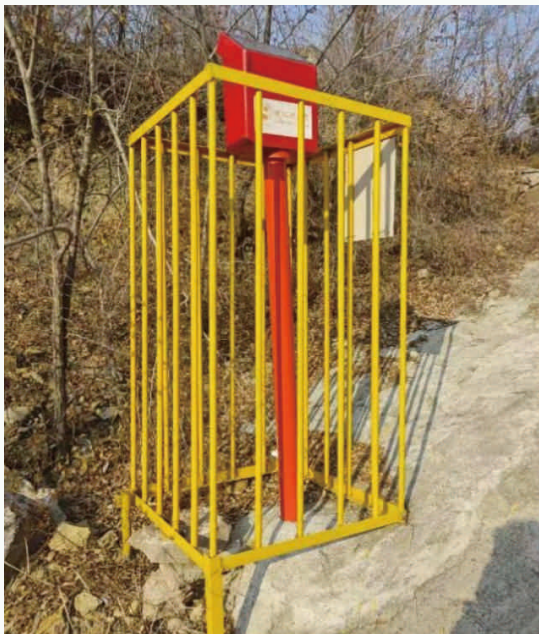
Overall Settlement and Stress Monitoring Points of the Project
