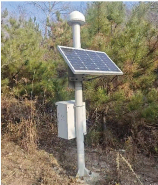
Overall Settlement and Stress Monitoring Points of the Project
