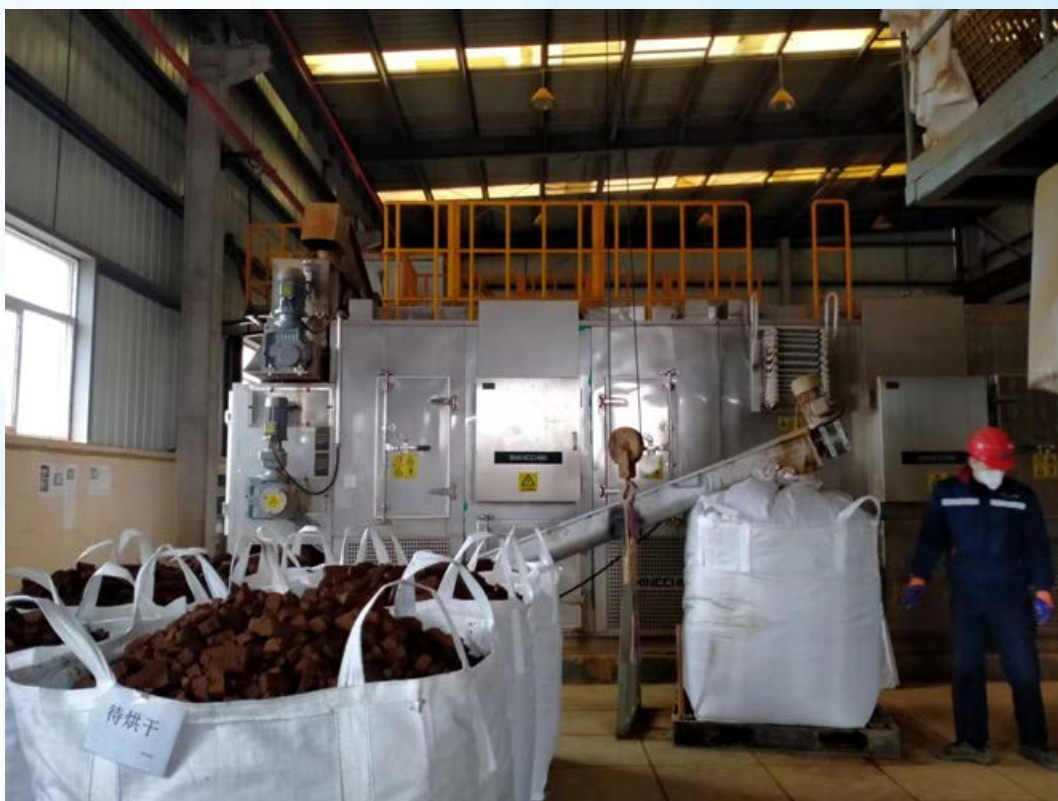
Figure 4 Low-temperature sludge dehydration equipment at Zhenjiang Sinotech 圖4 鎮江華科低溫污泥脫水設備
